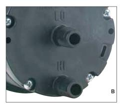
A- The standard Minihelico II gage is supplied with two barbed pressure taps molded into the rear housing of the gage. These connections allow easy, fast connection to the gage using 3/16" I.D. rubber or plastic
