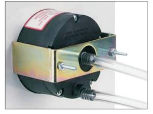
Mounting hardware is supplied with the Minihelice II gage for panel mounting through a single hole, 2-5/8" (67 mm) in diameter. Panel thickness up to 1/2" (13 mm) can be accommodated with the hardware supplied. If necessary, surface mounting of the gage can be accomplished by means of two 4-40 screws into the tapped mounting bracket stud holes in the rear of the gage. Surface mounting requires clearance
